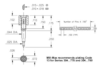
**Description:** Interconnect Socket Solderless Press-Fit Socket Accepts .015" - .025" (0,38 - 0,635 mm) dia leads Single Row Through Hole **Plating Code:** Shell Plating:
